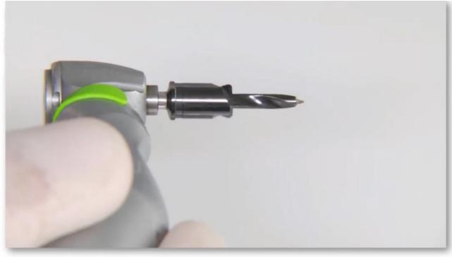
Choose the final length of the drill according to the length of the implant to be inserted.
